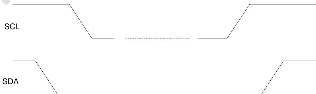
Figure 13: I 2 C START and STOP Condition Timing
