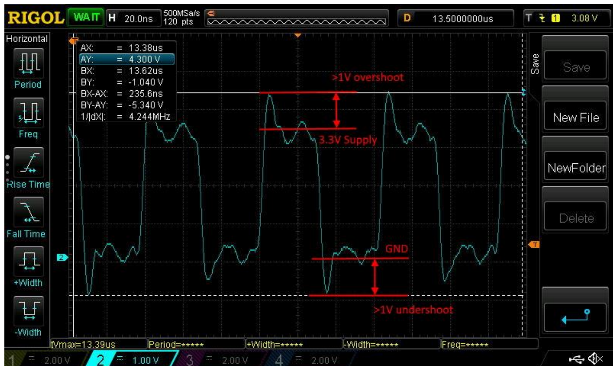
Figure 3: This trace image clearly shows the overshoot and undershoot present on the SPI lines were resulting in a peak-to-peak voltage of 5.65V, which exceeds the absolute maximum value documented in the Flash memory specification.
