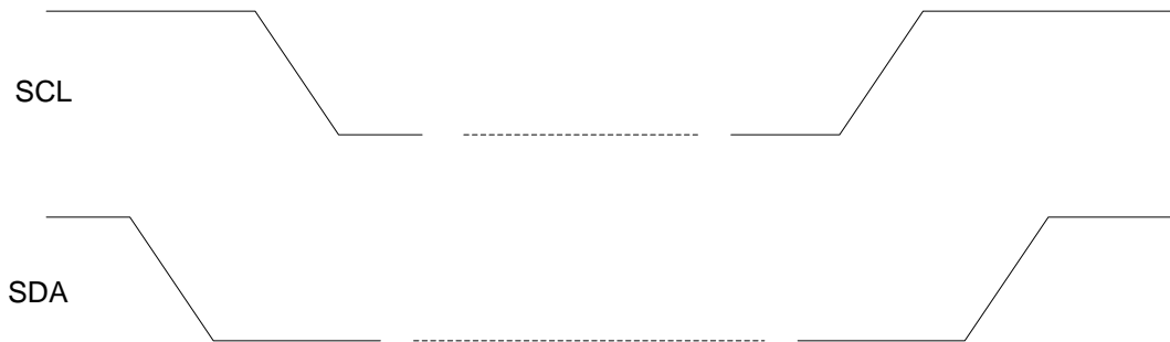
Figure 6: I 2 C START and STOP Condition Timing
