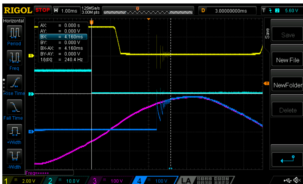
Figure 9: Measurement of the actual operation time of the relay
