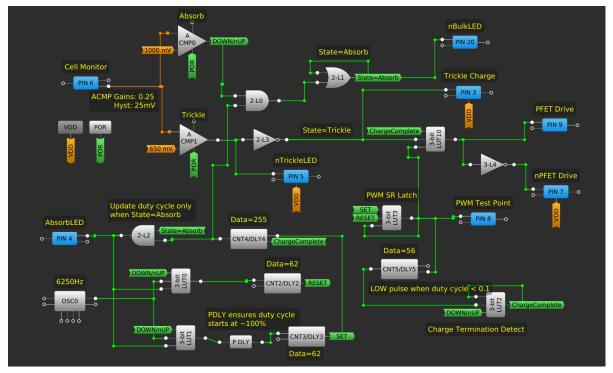
Figure 2: SLG46533V Designer diagram for the Li-lon charger
