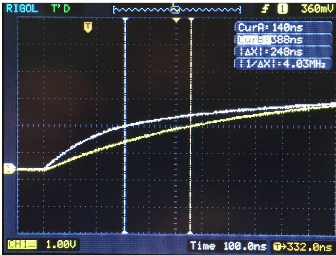
Figure 2: Oscilloscope Capture Showing the Difference in Risetime
