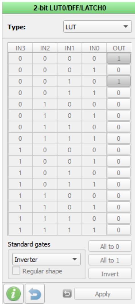
Figure 7: Bit Inverter
