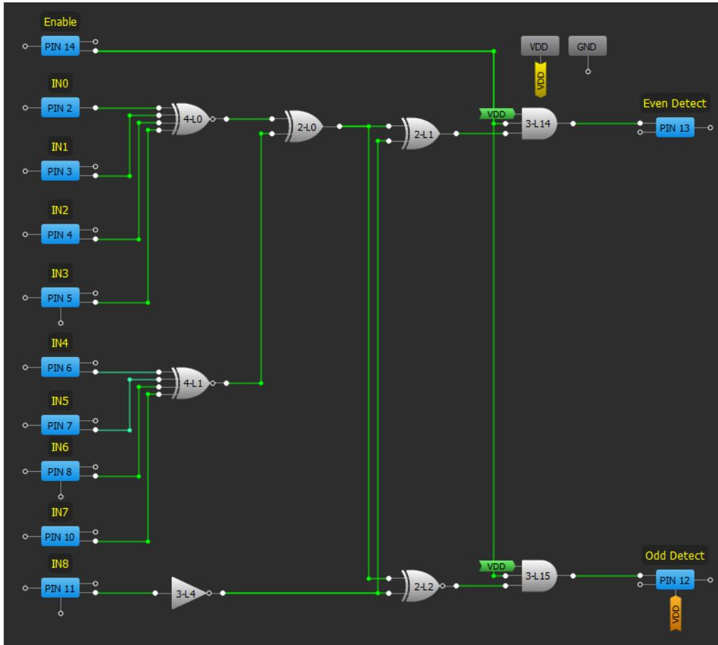
Figure 13: Parallel Input Parity Generator and Checker
