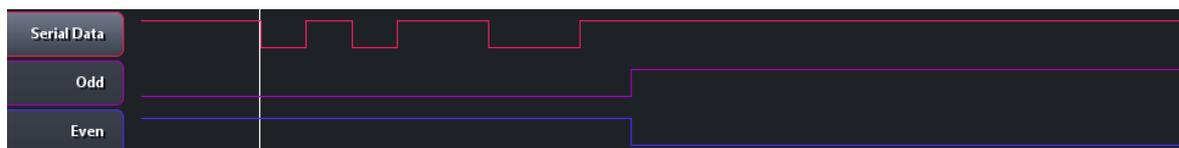
Figure 21: Serial Input Parity Generator Odd Test
