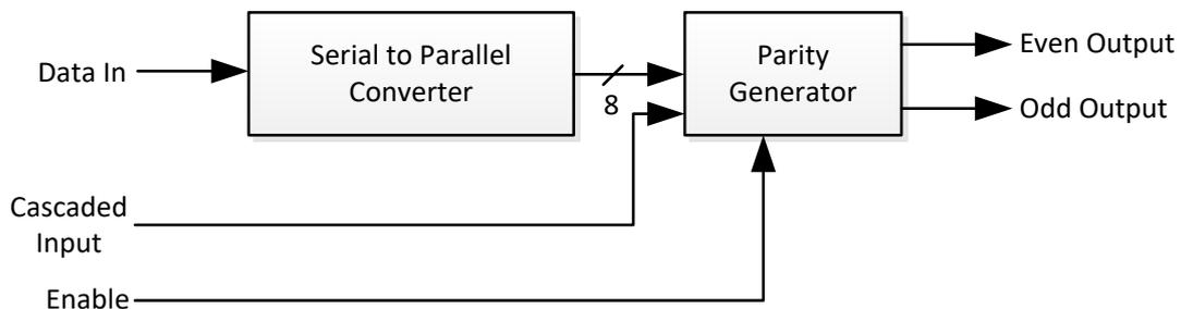
Figure 5: Serial Input Parity Generator Schematic Diagram
