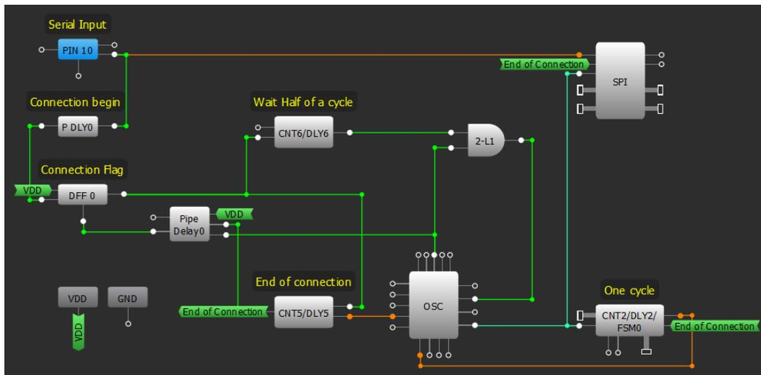
Figure 14: Serial to Parallel Converter (Matrix 0)
