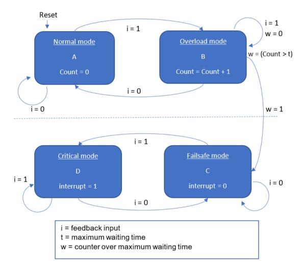
Figure 1: Flow or State Diagram of System
