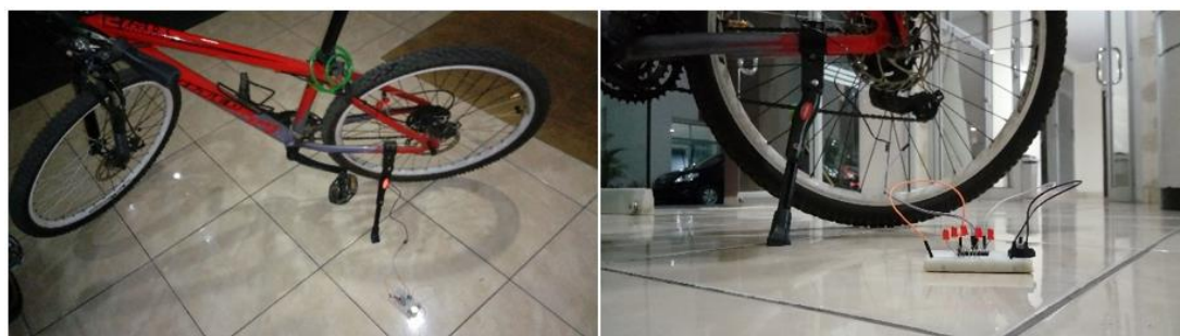
Figure 9: Magnet and Magnetic Switch Attached to Bicycle
