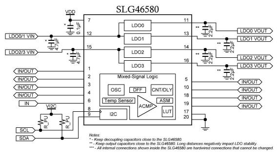
Figure 4: SLG46580 Typical Application Circuit ~ LDO Configuration
