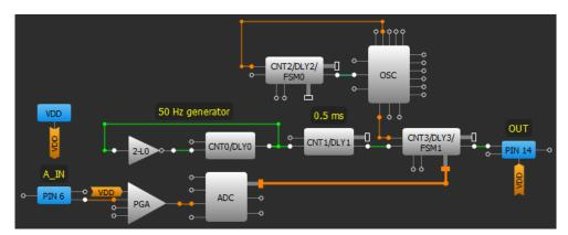
Figure 4: Design Implementation with GreenPAK
