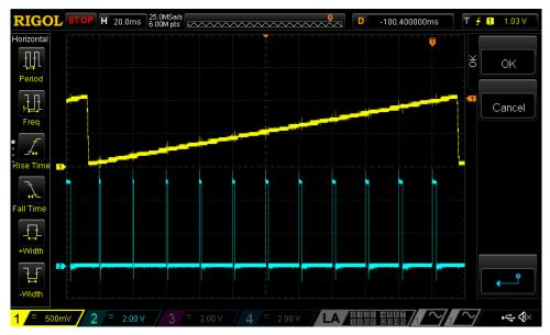
Figure 6: GreenPAK Design Operation Scope Shot
