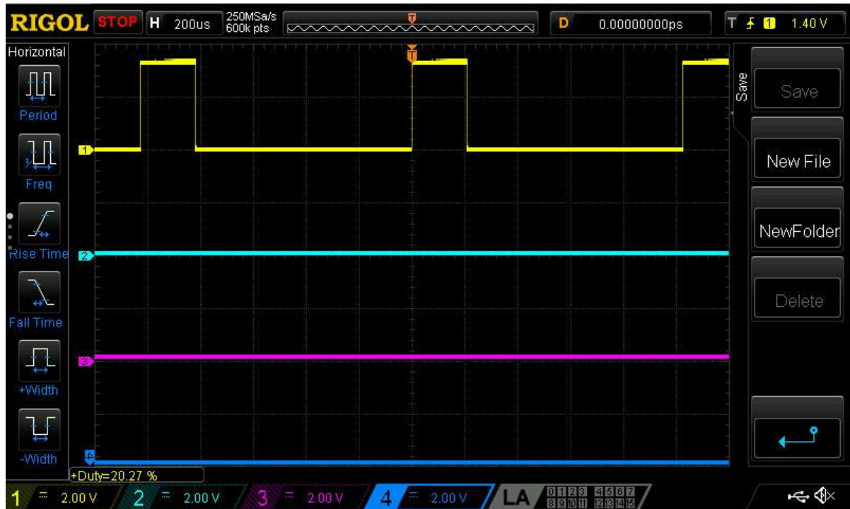
Figure 14: Minimum Limit of PWM Duty Cycle
