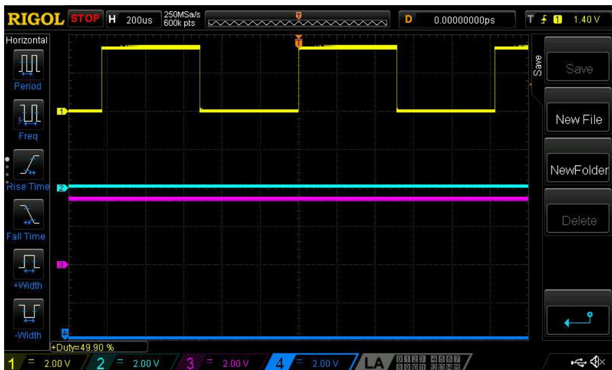
Figure 13: Maximum Limit of PWM Duty Cycle
