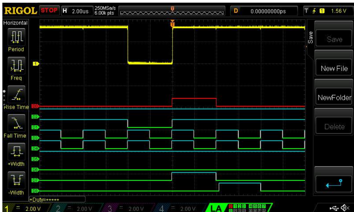
Figure 8: A Signal After Duty Cycle Has Become Maximum
