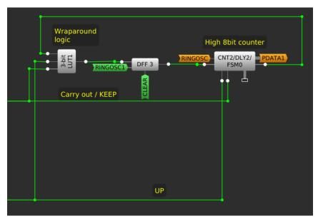
Figure 6: Wraparound Logic for High 8-bit Counter
