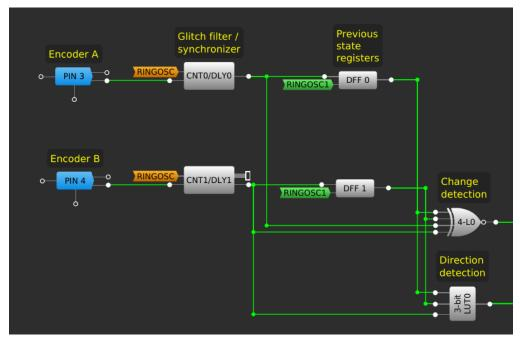
Figure 3: Quadrature Signal Input Block
