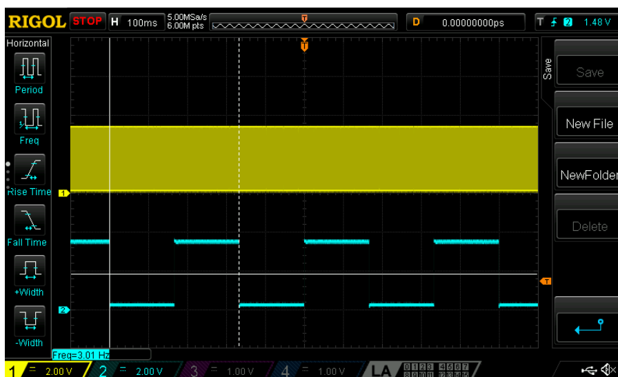
Figure 5: Square Wave while Constant Current Source is Enabled
