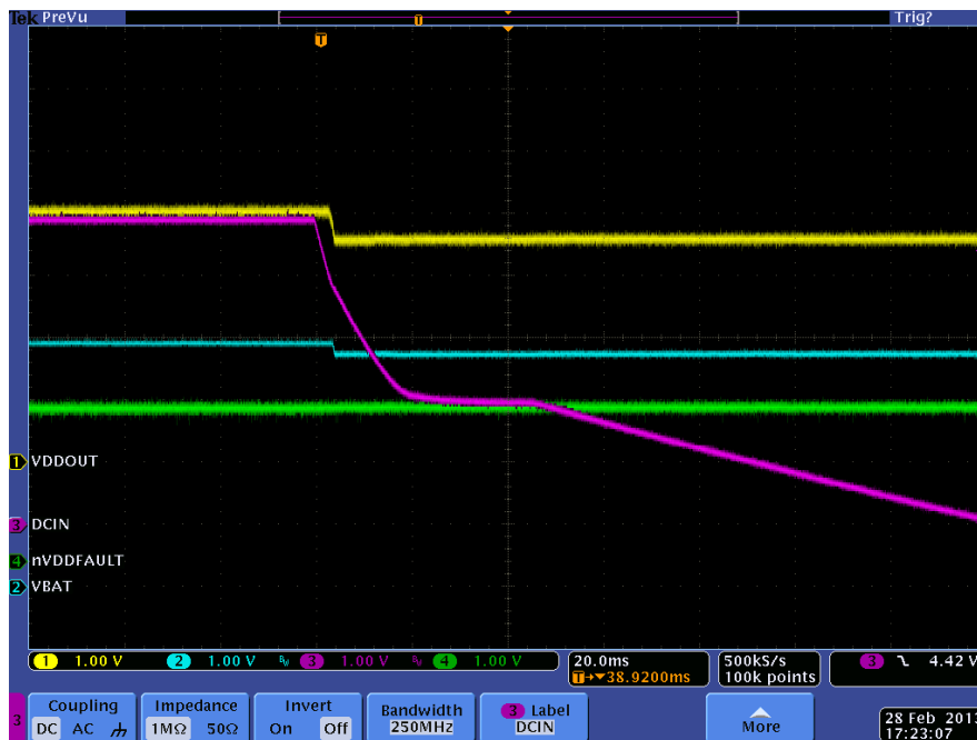
Figure 6 Supply sleep current via diode onto VBAT.
