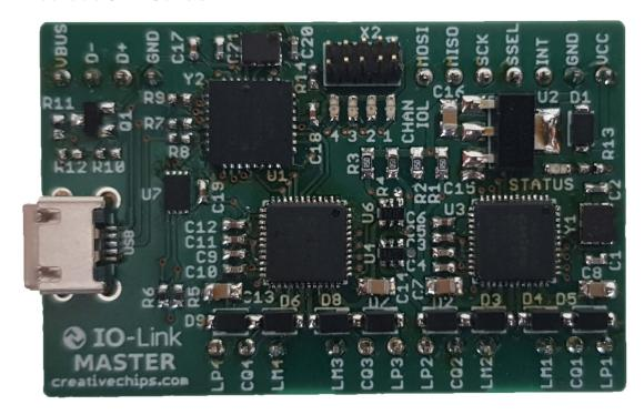
It is quick and easy to incorporate CCE4510 into an IO-Link system with the availability of a full evaluation board.
