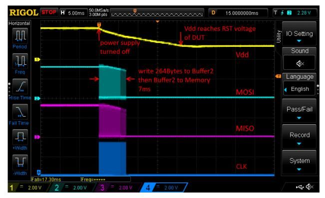
Figure 3. Oscilloscope Output of Experiment 1
