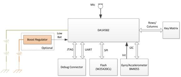
Figure 4: HW architecture of the Bluetooth Smart Voice and Motion Remote Control
