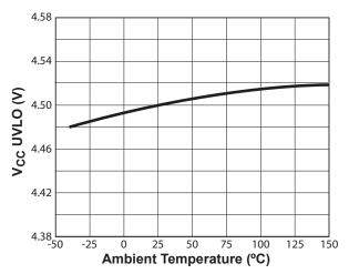
Figure 7.1 : V<sub>CC</sub> UVLO vs. Temperature
