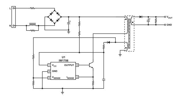
Figure 3.1: iW1706 Typical Application Circuit
