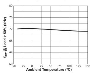
Figure 7.3 : Switching Frequency vs. Temperature<sup>1</sup>
