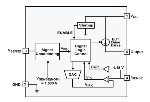
Figure 8.1 : iW1706 Functional Block Diagram
