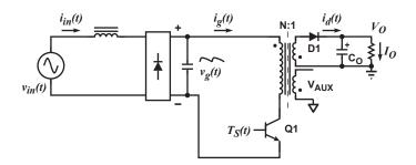
Figure 9.2 : Simplified Flyback Converter
