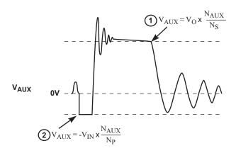
Figure 9.3: Auxiliary Voltage Waveforms
