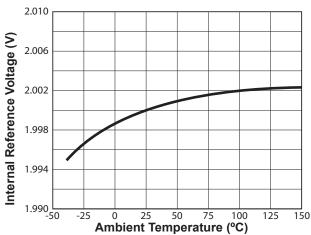
Figure 7.4 : Internal Reference vs. Temperature
