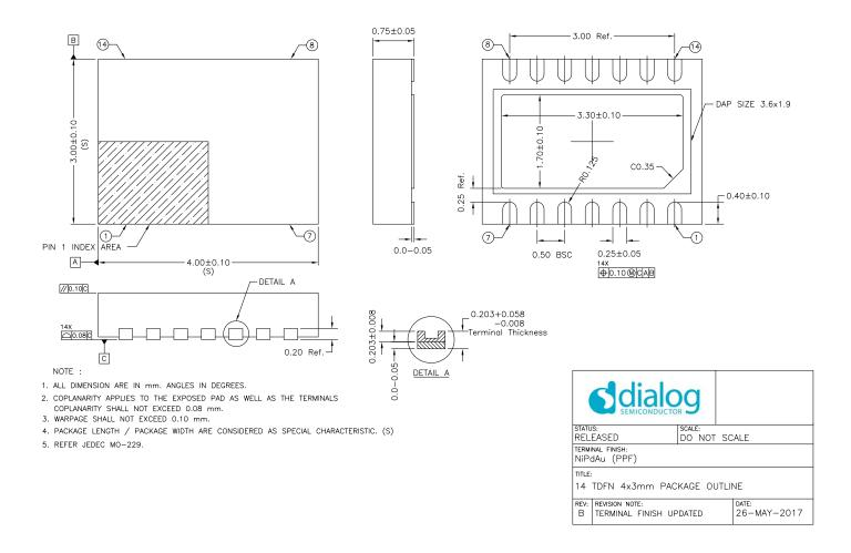
Figure 6.1: 14-Lead TDFN 4x3mm Package
