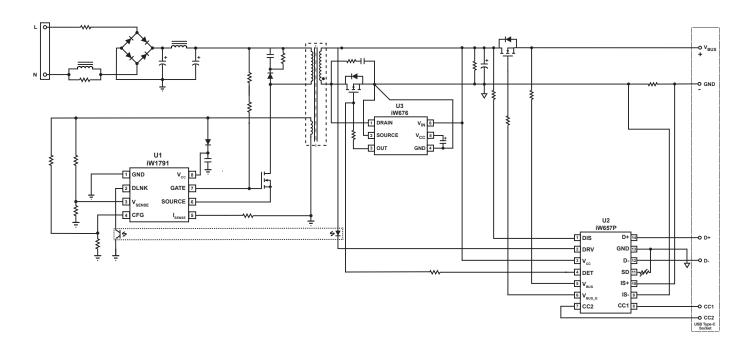
Figure 3.1: iW657P Typical Application Circuit with Secondary-Side Current Sensing (with iW1791 as the Primary-Side Controller and the iW676 as the Synchronous Rectifier Controller)
