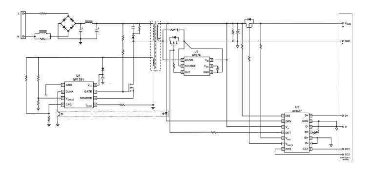
Figure 3.2 : iW657P Typical Application Circuit without Secondary-Side Current Sensing (with iW1791 as the Primary-Side Controller and the iW676 as the Synchronous Rectifier Controller)
