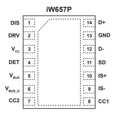
Figure 4.1 : 14-Lead TDFN 4x3mm Package (Top View, Transparent)
