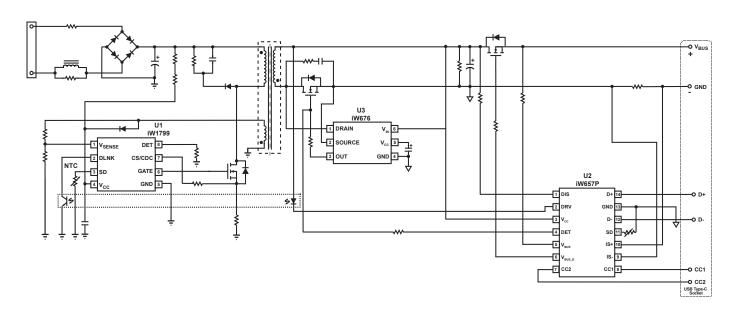
Figure 3.3 : iW657P Typical Application Circuit with Secondary-Side Current Sensing (with iW1799 as the Primary-Side Controller and the iW676 as the Synchronous Rectifier Controller)
