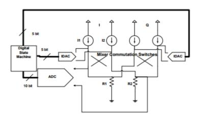
Block Diagram of the Calibration Scheme
