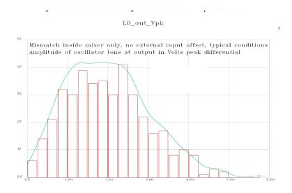
Monte-Carlo statistical simulation of mixer LO feedthrough showing Raleigh distribution
