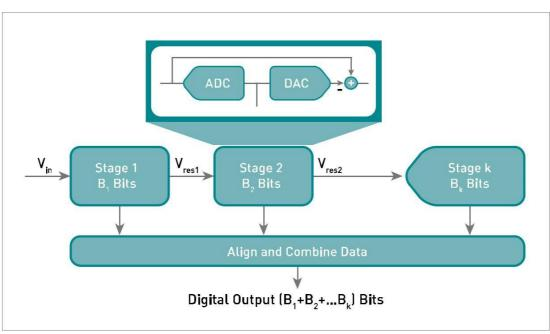
Figure 1. Pipeline ADC Block diagram
