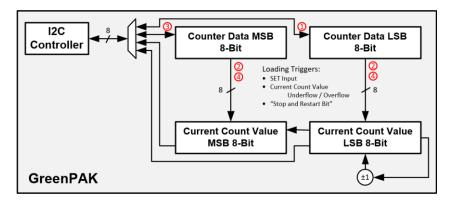
Figure 11: 16-Bit I2C Counter Block Diagram
