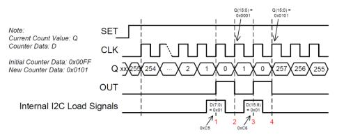
Figure 10: I2C Write of 16-Bit Counter Data Example
