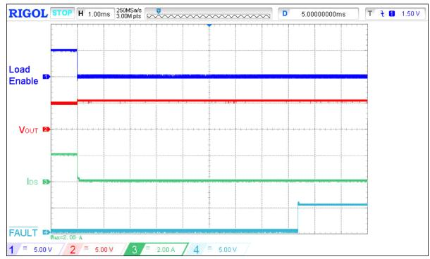
Figure 10. Typical FAULT de-assertion waveform for V<sub>DD</sub> = V<sub>IN</sub> = 5 V, C<sub>LOAD</sub> = 10  $\mu$ F, I<sub>ACL</sub> = 2 A, R<sub>SET</sub> = 40 k $\Omega$ , switch out 2  $\Omega$  load
