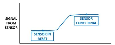
Under the correct conditions the Oversampling and Averaging technique described previously can be employed to provide further noise reduction. In this scheme, multiple measurements are taken of both the reset level and the signal level, the resulting output is the difference of the average of the signal measurements and the average of reset measurements.
