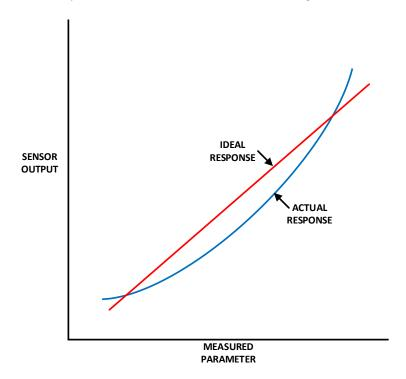
With sufficient measurements the curve-fitting coefficients for the characteristic curve of the sensor can be calculated. Those coefficients feed into the linearization formula used to compensate for the errors in the sensor measurement.
