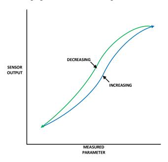
If the hysteresis effect is tolerable a single characteristic curve for the nonlinearity can be determined that is a close fit to both curves and used to derive the linearization formula for the sensor.
