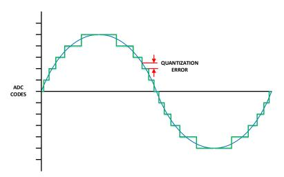
The magnitude of the quantization error is inversely proportional to the chosen ADC resolution (e.g. 12-bit). Increasing the resolution is one way of improving the accuracy of the quantized signal but there are diminishing returns as the complexity of the ADC increases significantly.
