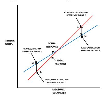
The measured parameters corresponding to both calibration reference points can then be used to compensate for the offset error and gain error of subsequent measurements. The following calculation is used to correct the sensor sample measurement:
