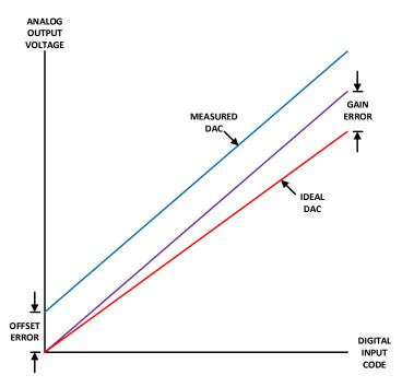
In some cases, the DAC output will go through some form of analog signal conditioning that may allow compensating for the offset error and gain error.
