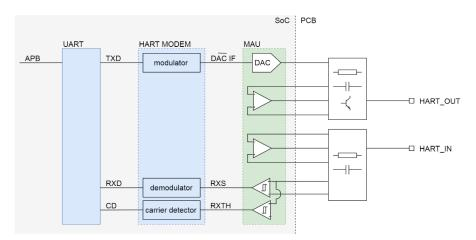
The list of parts that remain outside the SoC is thus reduced to passive components for filters that extracts FSK signal from the current loop and passive components and bipolar transistors that superimpose the output FSK signal to the current loop signal.
