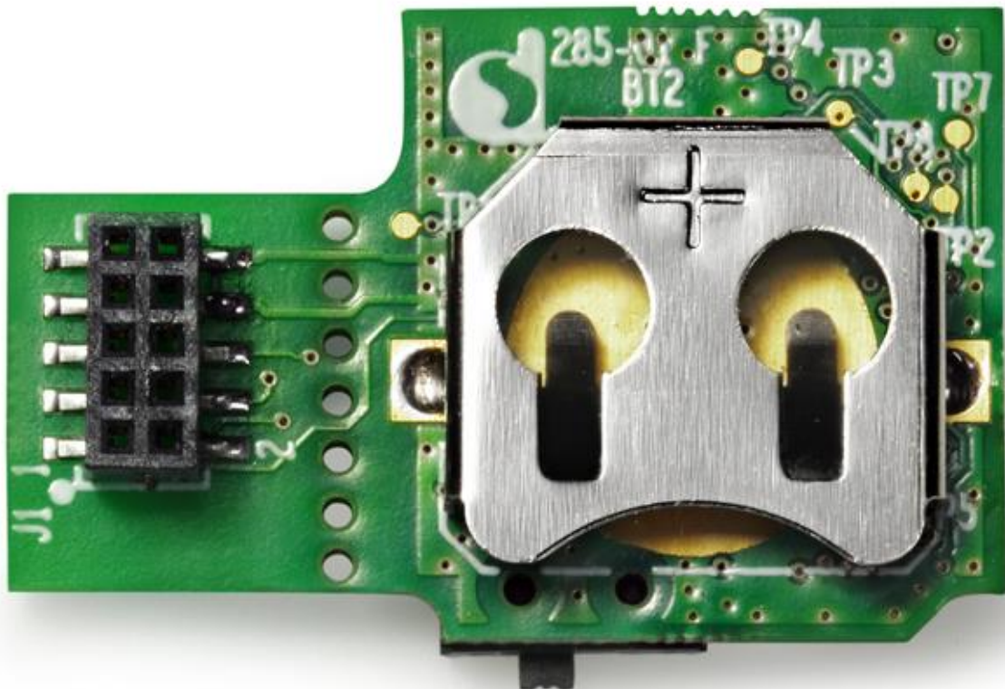
Figure 12: IoT Sensor reference board (bottom view)
