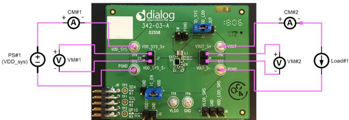
Figure 4: Recommended Setup for Buck Efficiency Measurement
